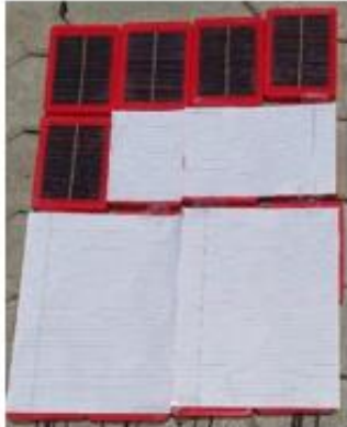
Fig 6.3 LW shading on HC configuration
