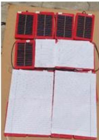
Fig 6.5 LW shading on MS configuration.
